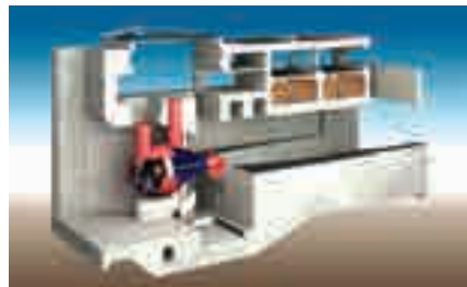
Cross-section of the tidal power turbine generator
