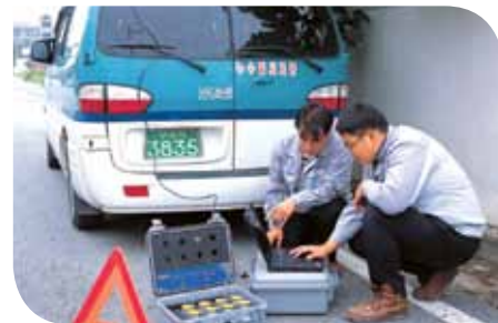
Water leakage inspection
